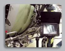
Borescope Inspection with JT8D On-wing Blade Blending
